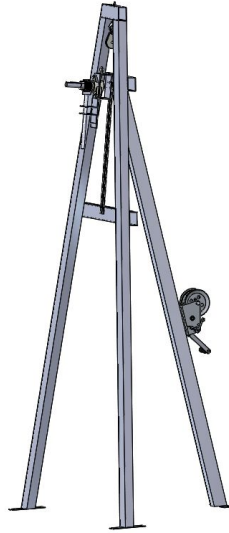
Figure 1. Guide Rail / Winch Design Change
